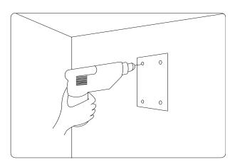
• Fix the bracket to the wall using plugs, taking care to leave the cables exit in the center between the fixing holes.
