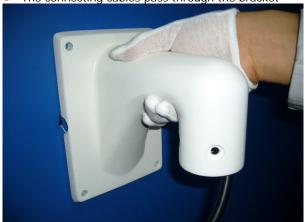
Connect the camera and secure it to the bracket with the supplied screws.
