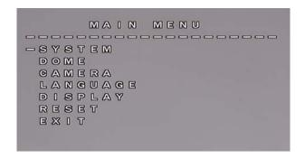
2 - Move to DOME with the up and down arrows, then press the right arrow to enter the dome menu
